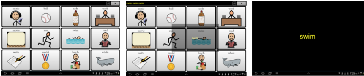
Figure 1: Example of the dynamic text feature within the graphics-based AAC grid display within the NOVA Chat 12. Upon selection of the graphic symbol with static text label (image on left), the text alone zooms out from the graphic symbol (image in the middle); the text then fills the screen for 3 seconds and the word is spoken (image on the right) before fading back into the graphic symbol. Refer to https://tinyurl.com/merc-on-aac-T2L for a video demonstration of the feature
