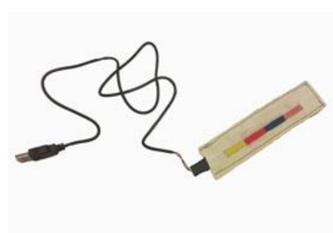
Figure 10 - The SoftPot sensor with four colors corresponding to different emotions. The SoftPot was also made to be easily connected to a laptop through a universal USB type A connection.
