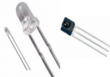
Figure 3 - Infrared Sensor, Transmitter, and Receiver
