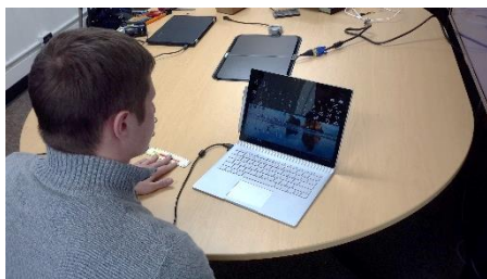
Figure 9 - Matt Vincent is demoing the use of our SoftPot membrane sensor integrated into the open source speech generation software, Optikey.
