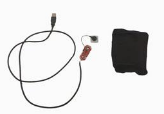
Figure 7 - The MyoWare sensor was designed to easily plug in to any computer using a universal USB type A. The black sleeve pictured, provides coverage and holds all sensor close to skin.
