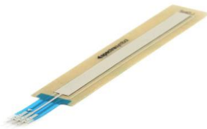
Figure 2 - SoftPot Membrane Potentiometer
